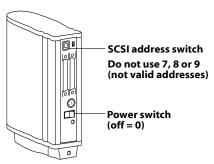
**Note:** The address is preset to 4. Do not change it unless another device is using 4. Other addresses typically available are 2, 5 and 6.
